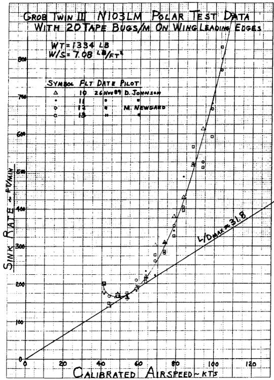
leading edges roughened with our standard pattern of 20 duct tape “bugs” per meter of wingspan. The wing drag probe data for that configuration are included in Figure 5, where large 8 to 12 knot drag increases are shown, compared to clean wing readings. It is quite apparent that even modern training sailplanes need to have their wings cleaned frequently for optimum performance.
