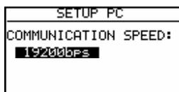
The new Windows PC program **Lxe** is able to **adapt the communication speed automatically**. The old DOS programs (LXGPS and LXFAI) are not able to do that.
