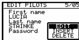
The function **INSERT** allows adding of more pilots (Up to 30). The message Active (upper right corner) indicates that specific settings of th shown pilot are active (means that this pilot has been chosen in the startup procedure).
