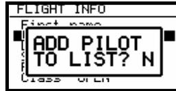
Confirming with Y(es) stores the pilot into the pilot list, what means this pilot can be chosen during the start-up procedure.
