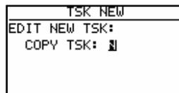
Using **Y** it is possible to copy any task from the TSK memory. After **N** the pilot should select all necessary turnpoints using the method described above.
