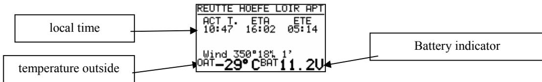
ETA (estimated time of arrival) and ETE (estimated time enroute) define the arrival time and the time needed to reach the target. Both depend on the settings in the INIT-menu. If there is no way to reach point (track and bearing differ more than 90°) both times will be replaced with stars. If the windcalculation is not active (depending on the method) the age of the last windupdate in min is displayed right of the wind.
